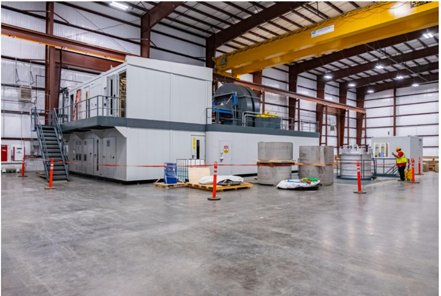
of an extremely high pressure at approximately 85 percent of the melting point of a metal, which allows the material to plastically flow. The pressure and temperature are sustained for a predefined time with the purpose to eliminate internal voids and defects in components or to consolidate powder to solid objects. The pressure and heat are applied uniformly to the components
